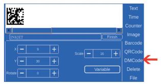
Click DM code  $\rightarrow$ Edit (input code content)  $\rightarrow$  Finish  $\rightarrow$  File  $\rightarrow$  Save or Save As Note: the size of DM code could be adjusted through Scale.
