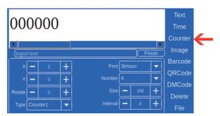
Click Counter to input serial number, set up type and size as need. One file could contain two different counters. Could set counter parameters in settings.
